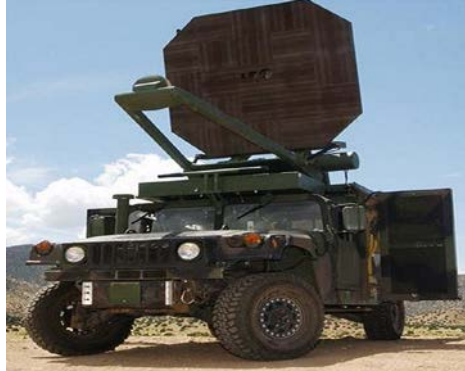
Fig.2. Active Denial System, used by US Army for crowd and perimeter control – a microwave NLW (wavelength 3.2 mm, frequency 95 GHz) which heating the epidermis of a target person to about 55°C.
